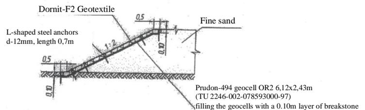
Figure 8 Structure of reinforcement of the subgrade berm's slope of the North Caucasian railroad
