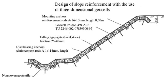
Figure 7 Structure of the slope of the railway subgrade
