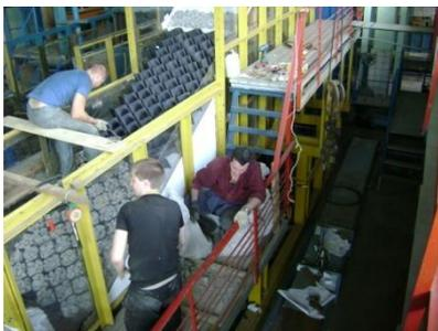
Figure 5 Mounting of stand for testing geocells with the filler which determines their level of erosion protection
