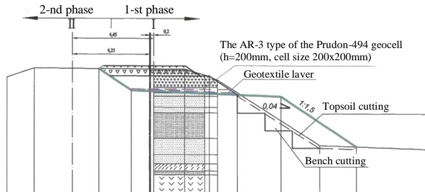
Figure 2 Railway line Minsk-Brest subgrade's structure
