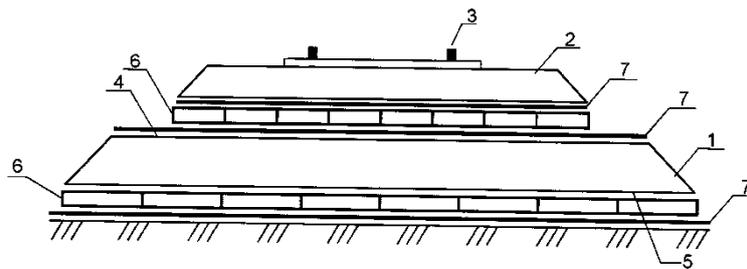
Figure 1 Structure of reinforcement of the railroad's foundation with plastic geocells
